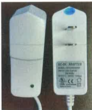
Incorrect 24V Power Supply
