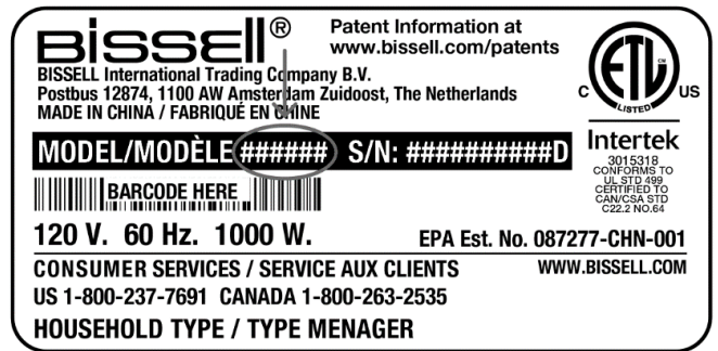
A close-up of the product rating label (model number location indicated by arrow)
