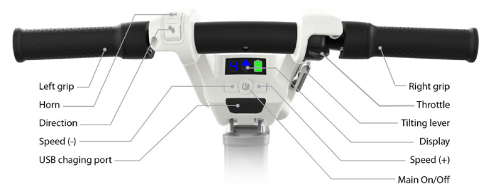
Figure 23 Driving Console overview
