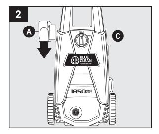
Slide spray gun holder (A) onto left side, when facing the unit, of power washer unit (C) as shown.
