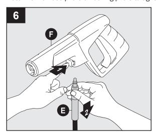
To release hose (E) from spray gun (F), press button on underside of gun toward trigger guard. The hose will slide out from connection.
