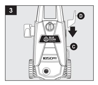
Slide cord hook holster (D) onto right side, when facing the unit, of power washer unit (C) as shown.
