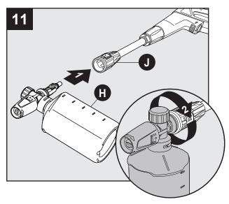
Insert detergent bottle (H) into extension lance (J), push in and turn clockwise
