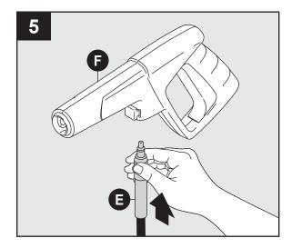
Connect the other end of high pressure hose (E) to spray gun (F) by inserting the silver metal tip of high pressure hose into the fitting just ahead of trigger guard. It will lock into spray gun with a "click". Confirm hose is locked into spray gun by slightly pulling on hose. The hose is now securely attached to spray gun.
