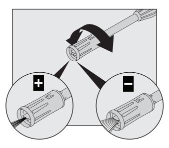
When using the variable spray nozzle, the spray pattern and intensity can be adjusted for each task by twisting the spray nozzle at the far end of the lance.
