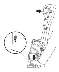
1 Plug power cord into outlet. Place foot on floor nozzle and tilt handle back.
