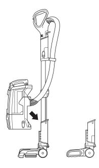
**3** To clean in upright mode, place pod onto wand and slide down to connect to the Dust-Away™ Pro.
