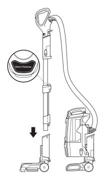
**1** Press Wand Release button to remove wand from motorized floor nozzle.
