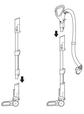
1 Place selected floor nozzle 2 Insert handle into wand. on floor and insert wand.
