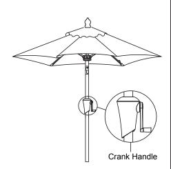
**Step 3:** Turn the crank handle in clockwise direction to open the umbrella canopy, turn the crank in the opposite direction to close canopy.
