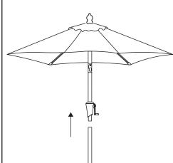
**Step 2:** Insert the bottom pole into the upper pole while pressing the snap button on the upper pole until the snap button locks into place.
