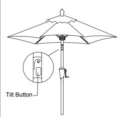
**Step 4:** Tilt the umbrella to the desired angle while pressing the tilt button to release the umbrella top. Release the button to maintain the desired angle.
