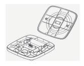
**Step 4:** Carefully open solar panel and set aside lid. Replace battery, matching the +/- on battery with the +/- on solar panel.
