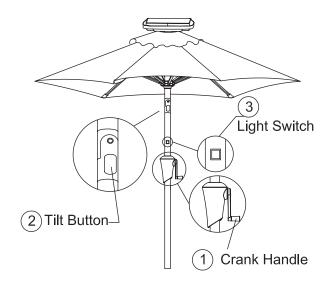
**Step 6:** Turn the crank handle in a clockwise direction to open the umbrella canopy. Turn in the opposite direction to close. You can tilt the umbrella to your desired angle by pressing the Tilt Button to release the umbrella top. Release the button to maintain desired angle. Press the fist light switch to turn on/off the regular LED function. Press the second light switch to turn on/off the moving lights function. Press the third light switch turn off the lights.
