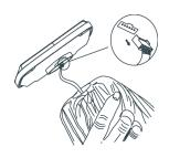
**Step 2:** Pull plug out of socket from under solar panel by holding plugs, not wires.
