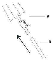
**Step 3:** To assemble the two pole pieces together, insert the bottom pole into the upper pole while pressing the snap button on the upper pole until the button locks into position.
