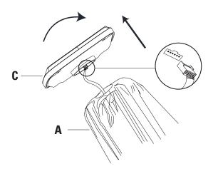
**Step 1:** Insert the plug into the socket under the solar panel.
