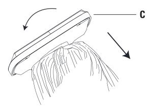
**Step 2:** Put the solar panel on top of the umbrella, and hide the plug and wire inside the groove at the top of the umbrella. Then turn the solar panel clockwise. Do not overtighten.
