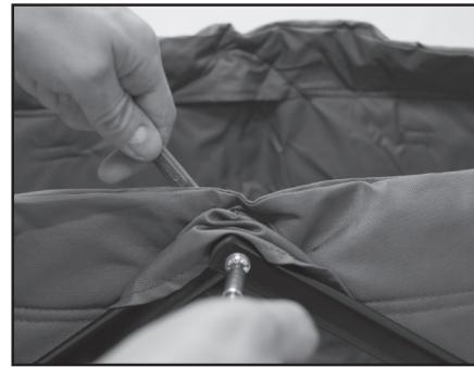
Using an H4 Allen Key and #10 wrench loosen and remove the nut on the inside of the wagon on both sides. Do not remove the bolt. It holds the frame together.
