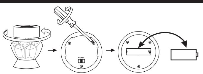
**BATTERY SPECIFICATION - BATTERIE SPÉCIFICATION - BATTERIE SPEZIFIKATION** 1 x AAA 1.2v Replaceable and rechargeable Ni-MH battery included.
