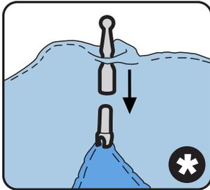
NOTE: Removable Truss Tips are designed to come off. If tips happen to come off, simply reattach as illustrated.
