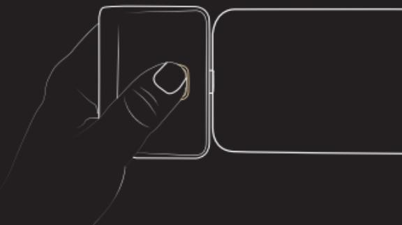
Re-insert the adapter into the TotalBoost Mini and apply pressure on the Switch while disconnecting from the device. This will hold the adapter in place.
