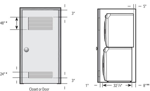
Required Dimensions for Installation with Stacking Kit
