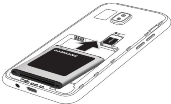
1. Insert the battery into the opening on the back of the device, making sure the connectors align.
