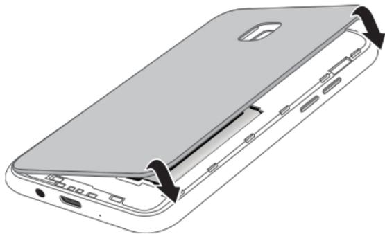
1. Place the back cover onto the back of the device and press down.
