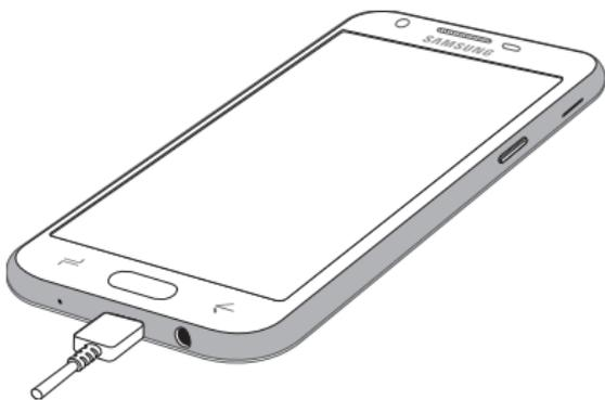
2. Connect the USB cable to the charging head, and then plug the charging head into a standard outlet.
