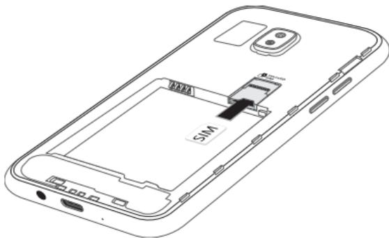
2. Slide the memory card into the slot with the gold contacts facing down.
