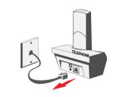
Insert the Line Cable into the LINE port of the Call Blocker.
