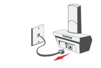
Insert the Line Cable into the **LINE** port of the Call Blocker.
