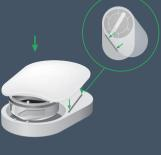
Insert the clip gently into the base by aligning the edge of the clip with the diagonal line on the base.
