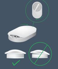
Twist the clip into place so that it aligns with the base. Check to make sure that the clip is not askew.
