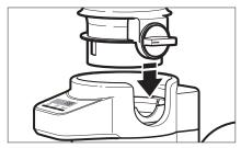
4. Install the ingredient hopper: Align the ingredient valve with the corresponding notch on the scale, and lower the hopper onto the scale until fully seated.
