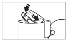
2. Install the sifter assembly: Lower the sifter into the sifter housing at an angle. Once the shaft is inserted into the sifter housing, press down on the back of the sifter to click it into place.
