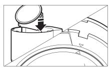
Install the swivel chute: Lower the swivel chute into the sifter housing at an angle, aligning the marks on the swivel chute with the marks on the inside of the sifter housing.
