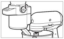
5. Before adding ingredients to the hopper, be sure the ingredient valve is in the closed position and swivel chute is pointed into the mixer bowl or an appropriate container.
