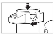
3. Install the scale: Place scale on top of sifter housing as shown, and slightly left of center. Twist the scale counterclockwise until it locks into place.
