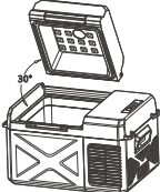
Prepare the door at a 30° angle
