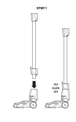
1 Insert the wand into the motorized floor nozzle connector until you hear a click.
