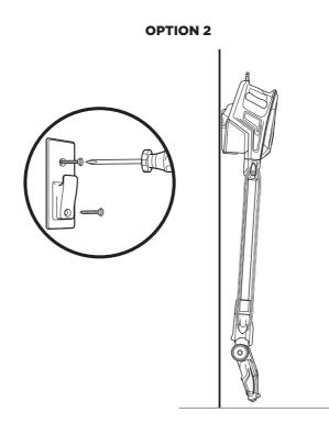
Use the wall mount that is included. Drill two 5/16" holes into the wall and insert the provided plastic anchors into the holes. Using a Phillips-head screwdriver, screw the wall mount into the plastic anchors. Hook the catch on the bottom of the handheld vacuum onto wall mount.
