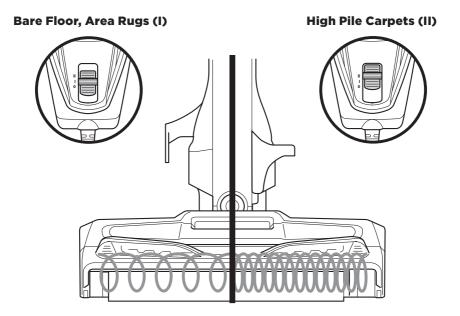
The Shark<sup>®</sup> Rocket<sup>®</sup> Complete with DuoClean<sup>™</sup> has a 2-speed power slider switch on the handle. Slide the power switch to appropriate speed setting (I or II) and start cleaning.
