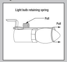
Pull away the bulb retaining spring, unscrew the old bulb, and replace with a new 40w candelabra bulb.
