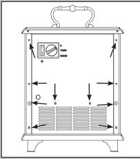
1. Loosen the Phillips head screws and remove back panel.
