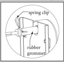
3. Pinch this spring clip to loosen. Gently turn and pull the rubber grommet of the motor shaft.
