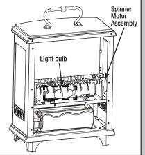
2. Remove back panel to access light bulb
