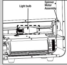
2. Remove back panel to access light bulb
