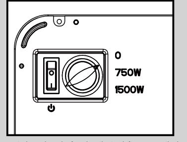
The control panel can be found on the top left corner on the back side of the unit.
