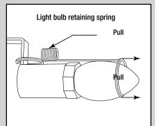
4. Pull away the bulb retaining spring, unscrew the old bulb, and replace with a new 40w candelabra bulb.
