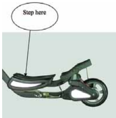
Figure 2: The front pedal should be depressed before pressing on the rear pedal.
