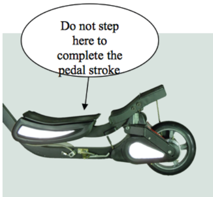
Figure: Pushing the rear part of the front pedal all the way down will make pedaling more difficult.
