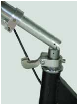
Figure: Pull out the steering column and fold the steering column down
