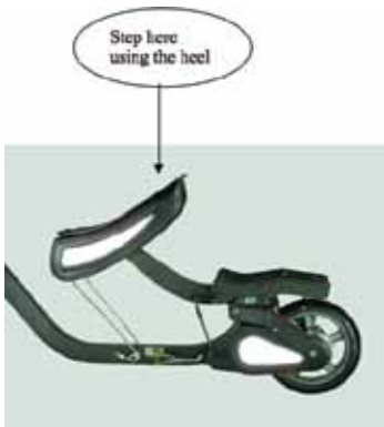
Figure 1: When pressing on the front pedal, use the heel. Then rock forward to the balls of the foot.
