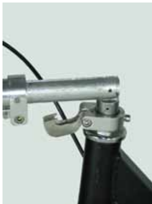
Figure: Pull out the steering column and fold the steering column down
