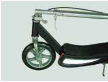
Figure: Turn the front wheel 180°
