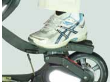
Figure: Correct position of the rear foot
