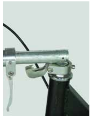
Figure: Pull out the steering column and fold the steering column down
