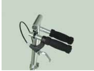
Figure: Handle bars should be folded towards the main body of the scooter
