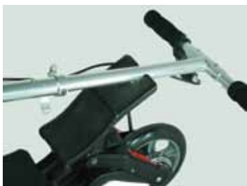
Figure: Hook the steering column to the back of the rear pedal by pushing the quick release button on the steering column to extend it.
