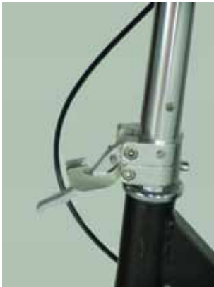
Figure: Open the folding lock lever to open the hook
