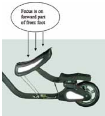
Figure 1: Press down on the front pedal with the forward part of the front foot and then press down on the rear pedal.
