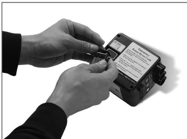
Figure 1: 9 volt batteries cover.
