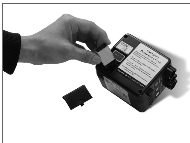
Figure 2: Install 9 volt batteries.
