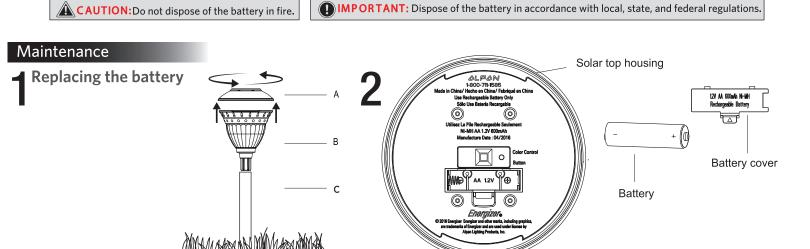
**Important:** Use only AA 1.2V 600 mAh Nickel Metal Hydride (Ni-MH) rechargeable batteries.
