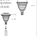
□ Insert the Solar Top Housing and Glass (A & B)
