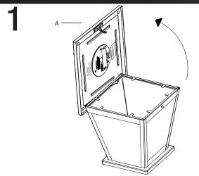
□ For first time use, remove pull tab from the battery compartment, located on the Solar top Housing (A).
