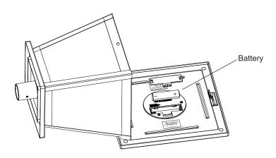
**Important:** Use only Lithium Phosphate 14500 (3.2V 600mAh) rechargeable batteries.
