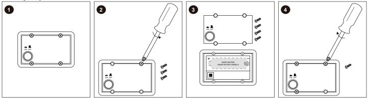
\*\* Battery type specified inside battery box. Replace with battery of identical specification. \*\*
