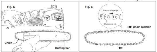
Starting at the tip, mount the chain drive links into the bar groove, leaving a loop at the back of the bar. The chain will loosely fit until it is placed on the sprocket. (Figs. 7 & 8) Make certain of the direction of the chain ➡→. If the chain is mounted backwards, the saw will vibrate abnormally and will not cut.
