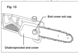
If the chain is too tight, it will not rotate. Loosen the end cover nut slightly and turn the chain tensioner 1/4 turn counterclockwise. Lift the tip of the guide bar up and retighten the end cover nut. Ensure that the chain can be rotated by hand without binding. A new chain tends to stretch; check the chain tension frequently, and adjust tension as required.
