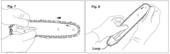
Hold the chain in position on the bar and place the loop around the sprocket. Fit the bar flush against the mounting surface so that the bar studs are in the long slot of the bar and the adjusting pin is in the chain tension pin hole (Fig. 9).
