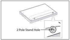
When using the wall mounting bracket, apply the adhesive protective label or protective cover to cover the unused stand openings. This will prevent the accumulation of dust and dirt. (Use only when provided with your particular model.)
