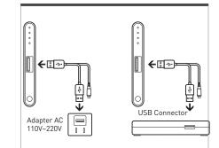
The battery indicator lights of XL 4200 will flicker one by one in direction of the arrow, indicating charging is taking place. When all indicator lights are fully lit, charging is complete.
