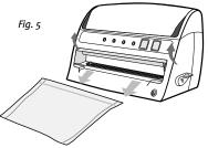
5. Lower door and lock side latch. Press Vacuum & Seal button (Fig. 4).
